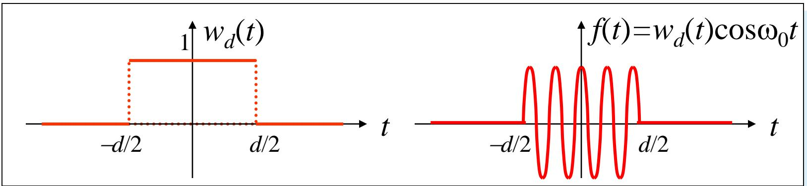
$$W_d(j\omega) = F[w_d(t)] = \int_{-d/2}^{d/2} e^{-j\omega t} dt = \frac{2}{\omega} \sin\left(\frac{\omega d}{2}\right) = \frac{1}{\pi f} \sin \pi f d = d \sin c \pi f d$$
