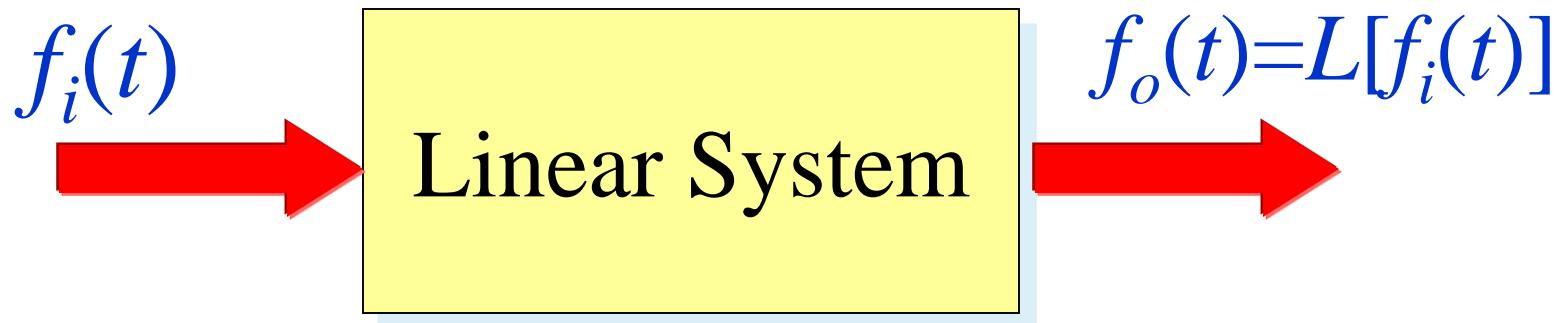
$$f_i(t) = a_1 f_{i1}(t) + a_2 f_{i2}(t) \rightarrow f_o(t) = L[a_1 f_{i1}(t) + a_2 f_{i2}(t)]$$
