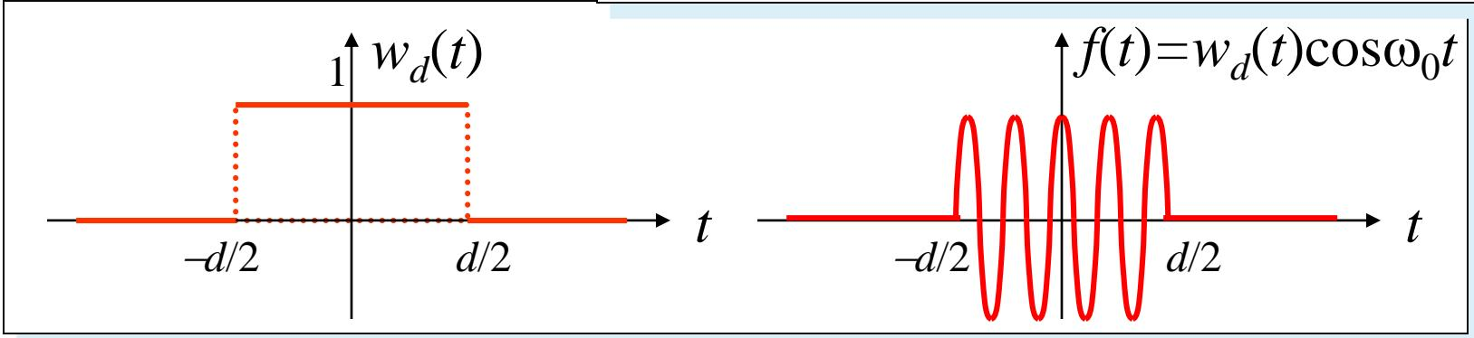
$$W_d(j\omega) = \mathcal{F}[w_d(t)] = \int_{-d/2}^{d/2} e^{-j\omega t} dt = \frac{2}{\omega} \sin\left(\frac{\omega d}{2}\right) = d \sin c\pi f d$$
