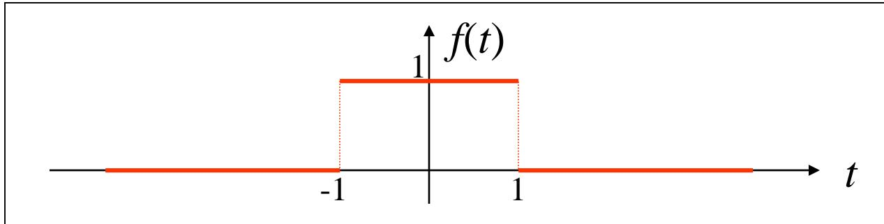
$$\begin{aligned} F(j\omega) &= \int_{-\infty}^{\infty} f(t) e^{-j\omega t} dt = \int_{-1}^1 e^{-j\omega t} dt = \frac{1}{-j\omega} e^{-j\omega t} \Big|_{-1}^1 \\ &= \frac{j}{\omega} (e^{-j\omega} - e^{j\omega}) = \frac{2\sin\omega}{\omega} = 2\sin c 2\pi f \end{aligned}$$
